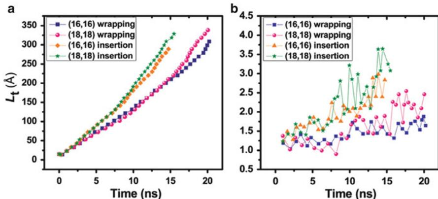
**Fig. 1.6** Variations of the ribbon length adhered onto the SWNTs  $L_t$  and the instantaneous velocities  $V_t$  against time during the GNR wrapping and inserting the SWNTs (16,16) and (18,18), respectively. (a) Ribbon length versus time and (b) instantaneous velocity versus time
