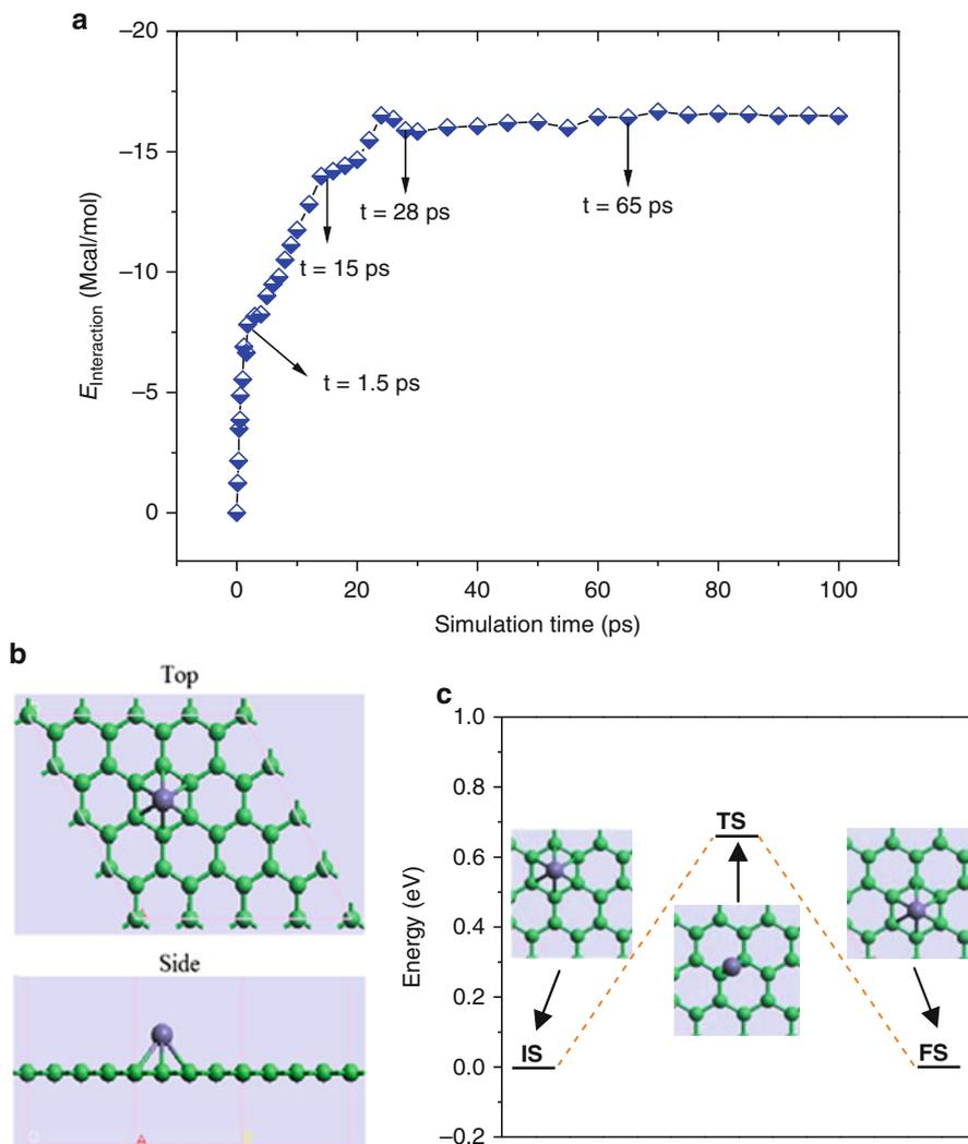
**Fig. 1.12** (a) The interaction energy between GNS and Fe NW with time. (b) *Top* and *side* views of the geometric structures of Fe adsorbed on GNS calculated by DFT. (c) Energy profile for Fe diffusion on GNS from one H-site to its neighboring one; the *insets* are the initial state (IS), transition state (TS), and final state (FS)
