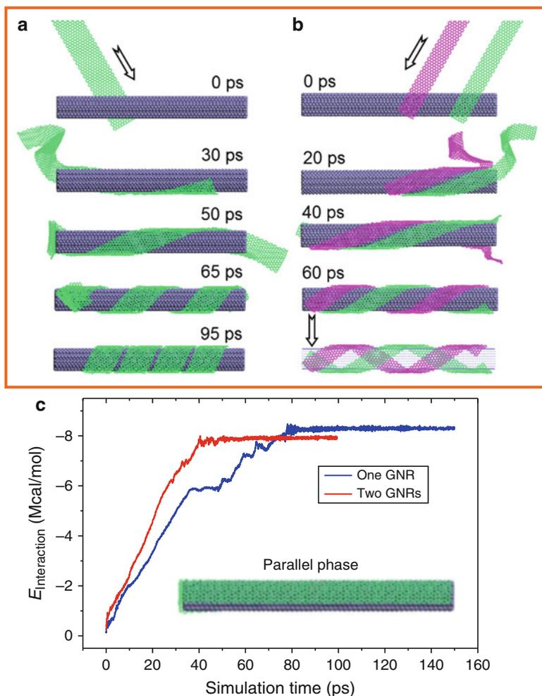
**Fig. 1.17** Snapshots of the helical rolling of one (a) and two GNRs (b) when placed at the angle of  $\varphi = 60^\circ$  with respect to the axis of the Fe NW. (c) The interaction energies between GNS and Fe NW during these two structural transition processes. The *inset* in (c) is the parallel phase of GNR on Fe NW
