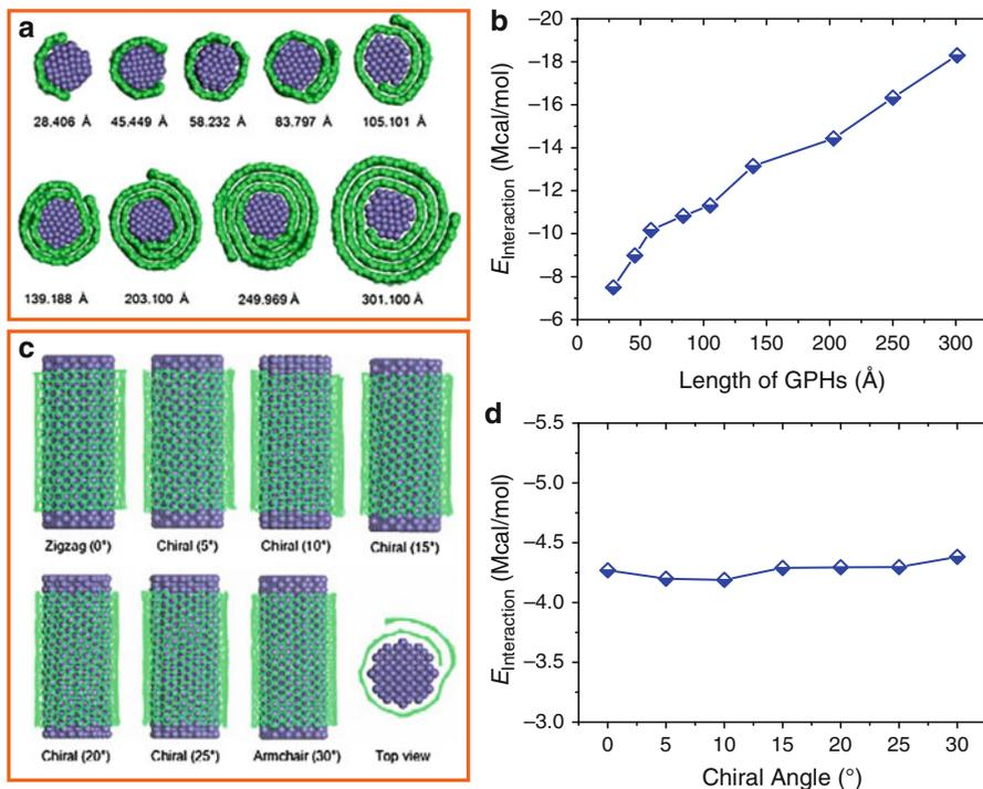
**Fig. 1.15** (a) The self-scrolling of GNSs with different lengths onto the Fe NW with same radius 6.4 Å and (b) the saturation interaction energies. (c) Different chirality GNSs wrapping onto Fe NW exhibit different chiralities and (d) the saturation interaction energies
