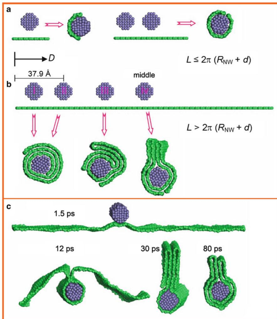
**Fig. 1.16** (a, b) Illustration of the position effect of the Fe NW on the self-scrolling of the GNS with different lengths and the final nanostructures. (c) A typical self-scrolling of the GNS onto the Fe NW located at the *middle*
