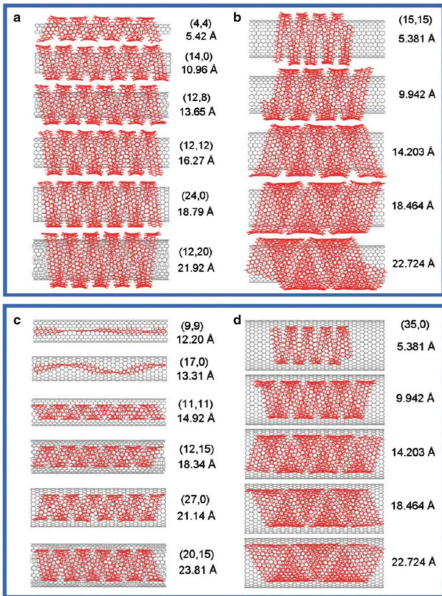
**Fig. 1.7** Dependence of the diameter and chirality of SWNT and the width of GNR in the helix-forming process. **(a)** Helical wrapping of GNR onto the SWNT with different diameters and chiralities, **(b)** helical wrapping of GNR with different widths onto the SWNT (15, 15), **(c)** helical encapsulation of GNR into the SWNT with different diameters and chiralities, and **(d)** helical encapsulation of GNR with different widths into the SWNT (35, 0)
