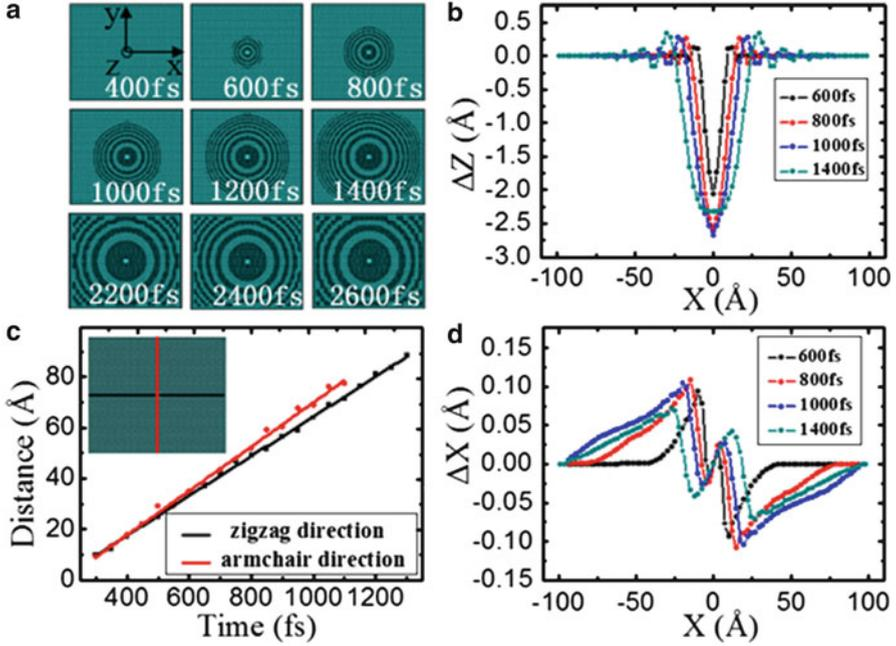
**Fig. 1.20** (a) The onset of the graphene ripple generated by striking with C60 molecule and its propagation on the surface of the graphene. The original ripples and the reflective ripples arouse interference pattern in the last three snapshots. (b) and (d) show the Z direction displacements ( $\Delta z$ ) and X direction displacements ( $\Delta x$ ) of atoms along the centerline [colored black in (c)], respectively. (c) The travelling distance of the ripples along different directions
