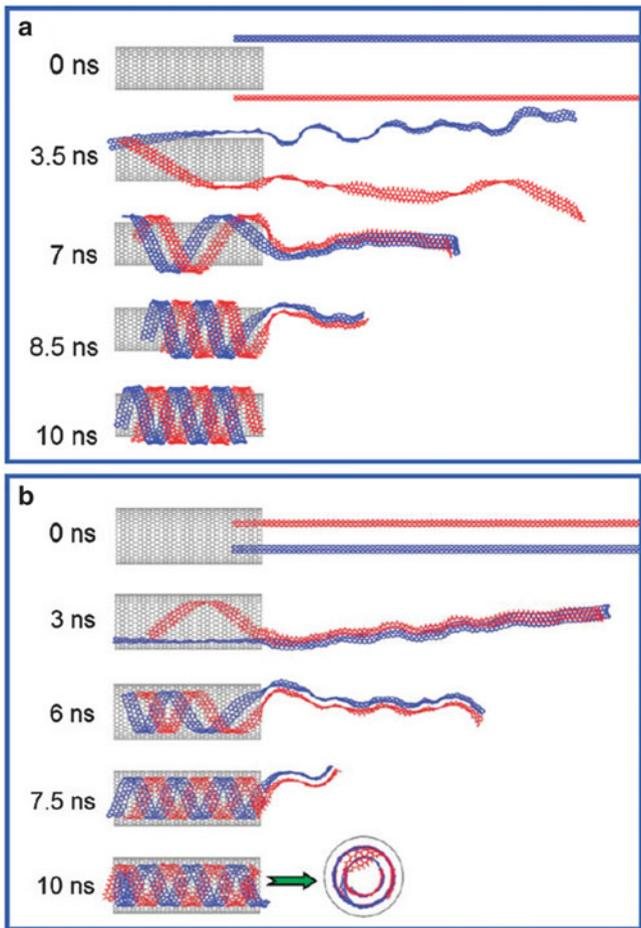
**Fig. 1.5** Evolution snapshots of two GNRs interacting with SWNT. (a) Helical wrapping of GNRs onto the SWNT (28, 0) and (b) helical insertion of GNRs into the SWNT (35, 0). The inset in part b is the top view of configuration at  $t = 10$  ns
