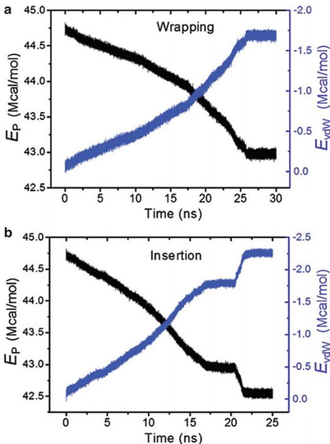
**Fig. 1.3** Potential energy ( $E_p$ ) of GNR-SWNT system and the vdW interaction energy ( $E_{vdW}$ ) between the GNR and SWNT as a function of simulation time: (a) helical wrapping and (b) helical insertion
