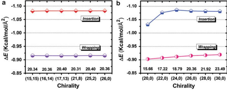
**Fig. 1.8** (a) Saturation interaction energies per unit area between the GNRs and the SWNTs with different chiralities. (b) Saturation interaction energies per unit area between the GNRs and zigzag SWNTs with different diameters
