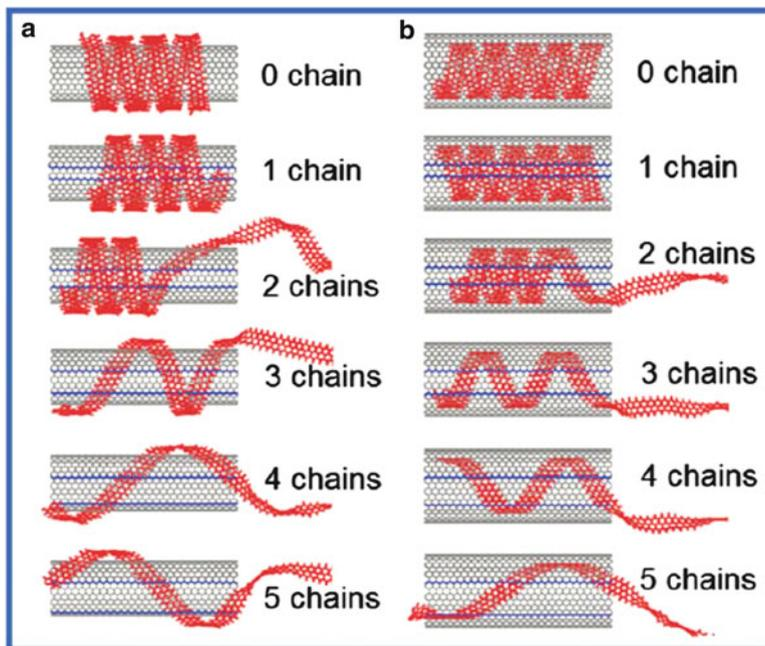
**Fig. 1.9** Effect of the gap of SWNT on the helix-forming process. The edges of gaps are marked *blue*. **(a)** Helical wrapping of GNR onto the SWNTs (15, 15) with gaps. **(b)** Helical encapsulation of GNR into the SWNT (20, 20) with gaps. *Insets* are the number of carbon atom chains that the gap contains
