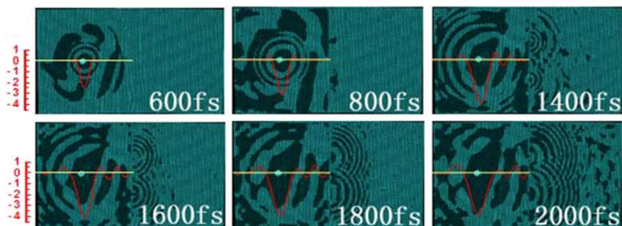
**Fig. 1.22** The propagation, diffraction, and interference of impacting ripples in the corrugated graphene. The inset *red line* of each graph is the *Z* direction displacements of atoms on the *yellow line*. Tick labels on the *left* are in unit of angstrom
